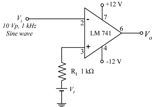
Fig 2. Circuit diagram of comparator
