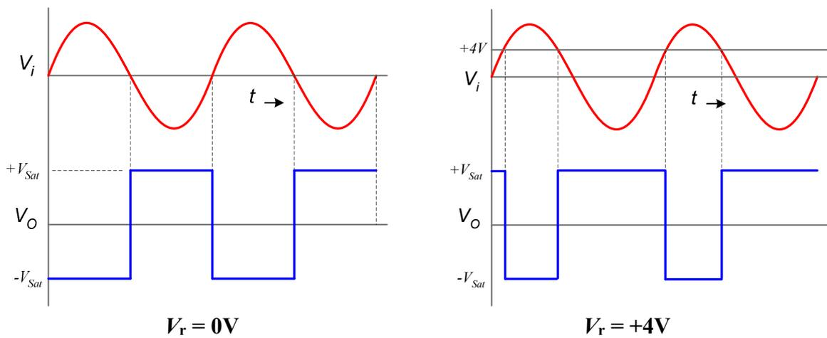
Fig 3. Waveforms comparator
