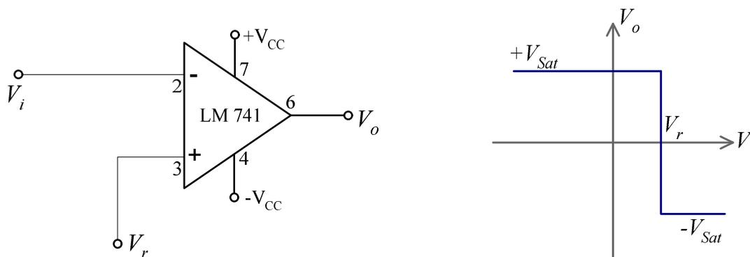
Fig 1: Comparator circuit and transfer characteristics
