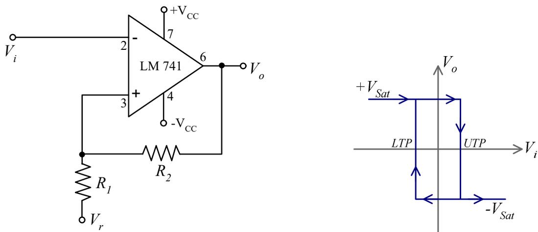
Fig 4: Schmitt trigger and transfer characteristics
